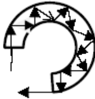
Fig. 1. Critical angle illustration and total internal reflection in plantain pseudostem fibre.
