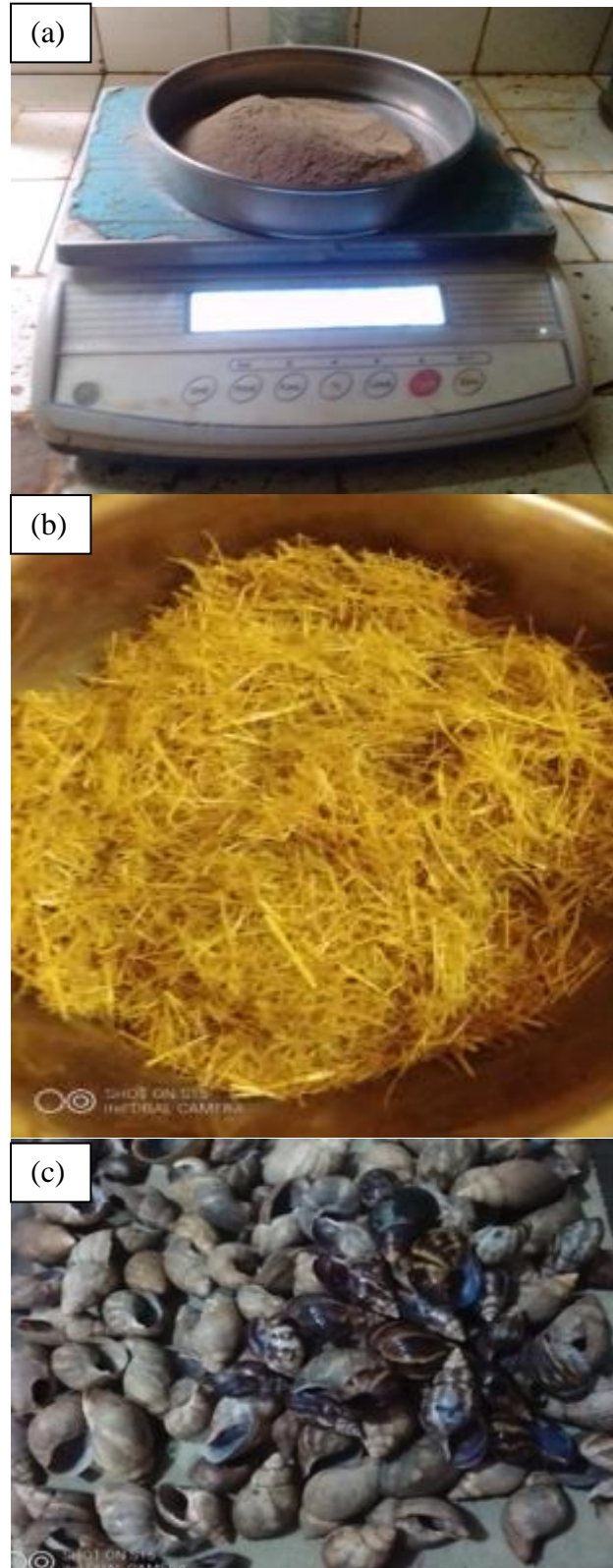
Fig. 1. Separate preparation of materials (a): weighing the soil, (b) Straw, (c): Snail shells.
