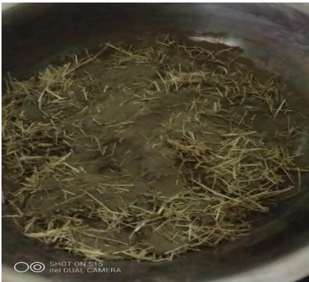
Fig. 2. Mixture of dry soil (earth), straw and provider snail shells.
