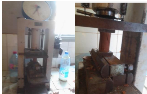
Fig. 5. Mechanical test apparatus, (a): Assembly of the parts, (b): Compression of the sample.
